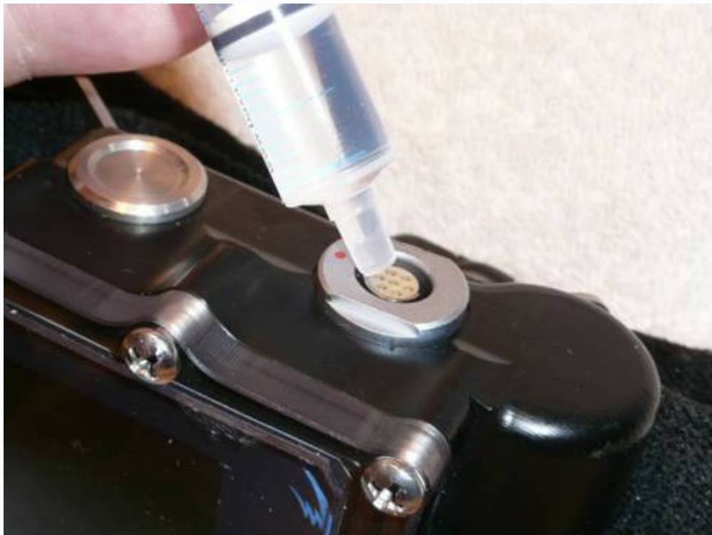
Adding Mineral Oil to Fischer Socket
