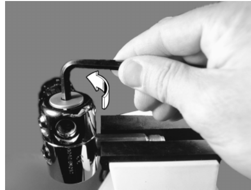
Figure 5 Removing Turret Retaining Bolt
