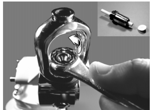
Figure 6 Removing Yoke Connector
