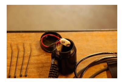
Battery housing: a 9V battery fits easy inside: make sure the cables do not clamp under the lid when closing the housing and don't tighten the lid hard when closing it: turn the lid till the end, and turn back a few degrees.
