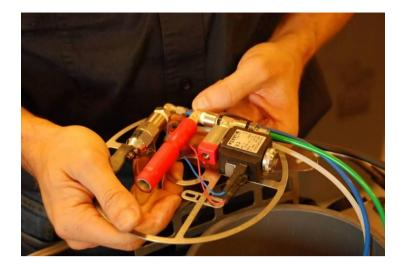
Connect the cable to the solenoid (polarity is not important), but make sure that there is no strain on the cables. (in this picture you can also see the thread of the solenoid outlet: if for some reason the solenoid would be blocked open, and you have no means of repair, you can block the outlet of the solenoid with the same plug as the orifice (same thread) and fly the unit manually! (pure mCCR) (if necessary remove part of the heat shrink of the solenoid outlet)
