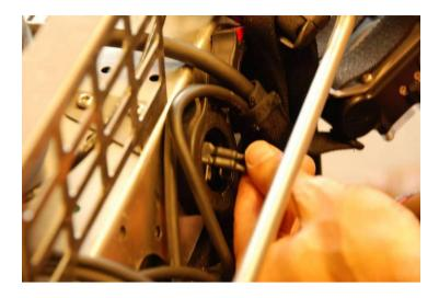
Insert the solenoid cable into the exhale lung, and...
