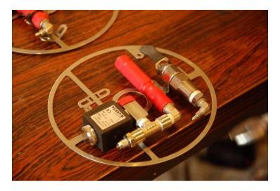
If after fixing and putting the lever horizontal, the connection to the tubing is not horizontal, you can adjust that by turning the connector round the thread with Teflon.
