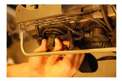
Now put the P-plug in place and feed the cable in.
