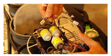
Connect the first splitter to cell 1, fit the side of the splitter with the protection (under the black heat shrink) to input 1 of the Pursuit, and the other side to input 1 of the first rEvodream (oxygen gauge side)
