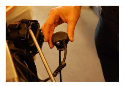
Now pass the cable with the connectors for the solenoid trough the P-plug of the exhale lung: un-tighten the cable gland completely so that the cable can move easy, put the connectors trough the hole and ...
