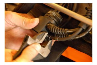
Tighten the lower part of the cable gland,...
