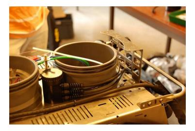
The battery housing in place, cables under the top grid.
