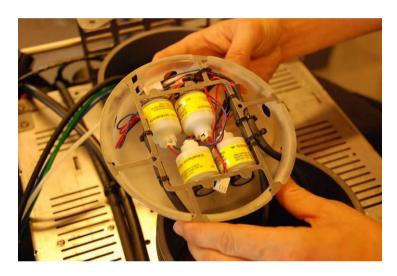
Put the plastic cell protection back in place, and make sure the molex don't tough the bottom of the plastic, where condensation can occur. If needed use a small tye-rap to keep them nice in place.
