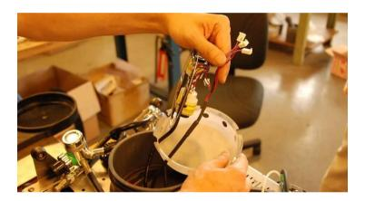
Feed the cable trough a free hole of the plastic cell protection, so that when the cell holder is in position in the inhale lung, the cable makes a clean curve.
