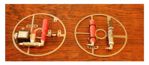
First thing: move the adv to the new solenoid grid; the old grid and orifice can be kept as spare, if you want to turn the unit back to pure mCCR.
