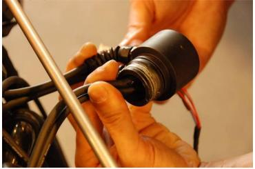
Pass the molexes one by one trough the hole of the P-plug ...
