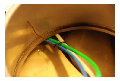
The cable, together with the 3 tubes must make a nice curve when the solenoid grid is placed in position: fix all 4 together as far as possible into the exhale lung, and when cutting the tyerap, make sure no sharp edges stay (if so use some sandpaper to smoothen the cut end). When installed in position, the cable/tubes may not interfere with the ADV!
