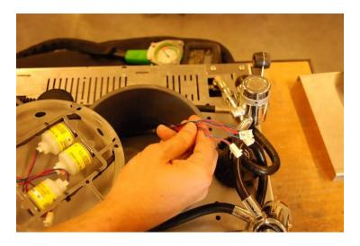
... and pull the cable till the inhale canister.
