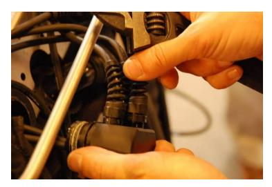
Now install the cable with the molex connectors in the inhale lung: if there is a gland-plug in
