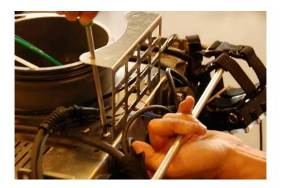
If they do not pass under the grid, loosen the bolts a bit so that the grid can be lifted. Don't loosen to much, or keep the screws in place with a finger trough the P-port of the inhale lung.
