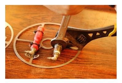
Use 2 wrenches to remove the ADV, and fix it on the new grid, making sure the 'lever' is horizontal!
