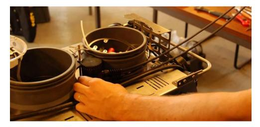
Now put the battery housing in place. The cable of the Pursuit runs around the exhale canister to the left shoulder, the cables with the molexes and connectors for the solenoid go under the protection grid on top of the unit.
