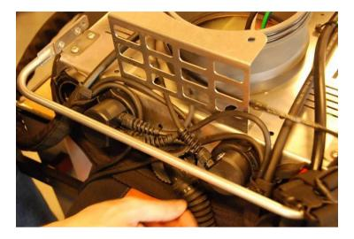
... feed the rest of the cable inside until the cable makes a nice turn towards the battery housing. (no strain on the cable). Now hand-tighten the upper part of the cable gland (verify the rubber seal is in correct position), and give it ¼ tour (not more!) with a key.
