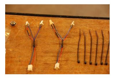
Cell splitters, the isolator each time on the left side in the black heat shrink: bottom side goes to cell, upper side left to pursuit, upper side right to rEvodream.
