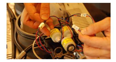
Connect the second splitter to cell 2, the side with the protection to input 2 of the Pursuit, and the other side to input 2 of the first rEvodream.
