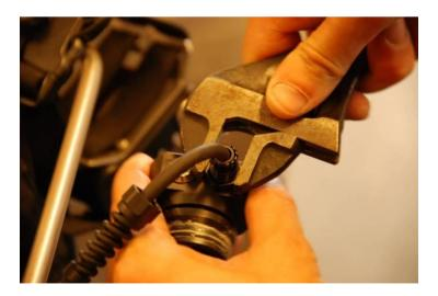
... tighten the lower part of the cable gland to the P-plug: for this you can use a wrench. Do **not** yet tighten the upper part of the gland, that fixes the rubber sealing. (you can see the rubber seal already in position)
