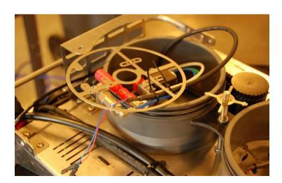
The solenoid cable can now be fixed on the grid, together with the white tube, with 2 tye-raps.
