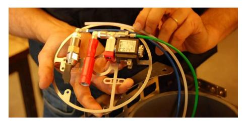
Now fix the green tube (oxygen) to the solenoid and the blue tube to the ADV. The fixing is done hand-tight + max 1 turn!
